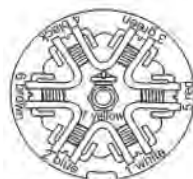
7-way trailer plug car end, rear view
