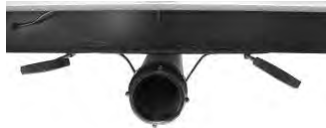
Black/Grey Tank Drain and Valves
