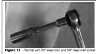
Figure 12 Ratchet with 3/8" extension and 5/8" deep well socket
